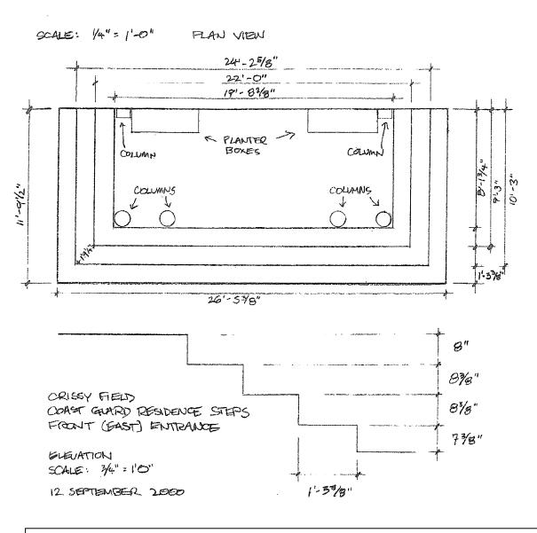
Figure 9: Sketch Plan and Section of the front porch, Building 1901, dated September 12, 2000, by GGNRA staff. Measurements indicate that it would be possible to provide an accessible entrance to the front of this building.
