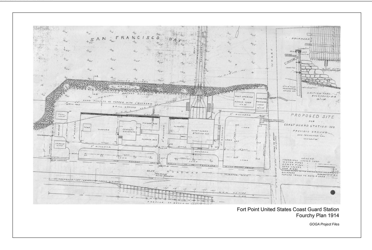
Figure 3: Fourchy Plan, 1914: In 1914, Andre Fourchy, Superintendent of Construction for the Life-Saving Service, drew plans for a new facility at a proposed site 700-feet west of the original lifesaving station location. Plans included a new two-story boathouse and dormitory, 55 feet by 55 feet. Fourchy completed the drawings by November of that year. (From the GGNRA Presidio Army Records Center.)
