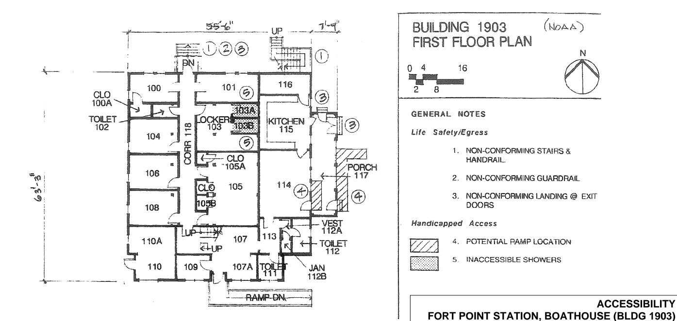
Figure 10: Access, Building 1903, First Floor Layout, ICAP Report, dated 1993, from the GGNRA park files. This ICAP Report documents current repair needs at the time of the survey. In 1993, the report indicated there was no handicap access provided at the Porch adjacent to room 117, and no ramp provided from room 117 to rooms 114 and 115. The ICAP report drawing illustrates one way to access the porch, which functions as a small museum, via an accessible ramp.
