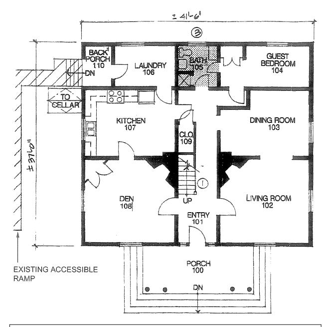
Figure 8: Building 1901, First Floor Layout, ICAP Report, dated 1993, from the GGNRA park files. This ICAP Report drawing documents repair needs at the time of the survey. In 1993, the report indicated there was no handicap access at the front porch and that it was inappropriate to provide building access from the laundry room. This access has remained unchanged.
