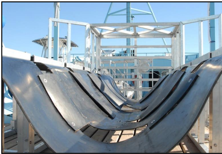
Fig. 8. Dr. Domeier's failed rubber-contoured shark cradle.
