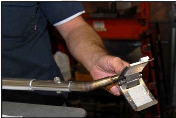
Fig. 9. Dr. Domeier's failed spring-loaded SPOT attachment device.
