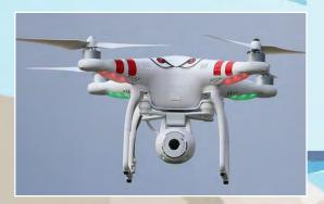
Unmanned Aircraft Systems or "UAS" include all unmanned craft: Unmanned Aerial Vehicles (UAVs), Remotely Piloted Aircraft (RPA) or "drones"
