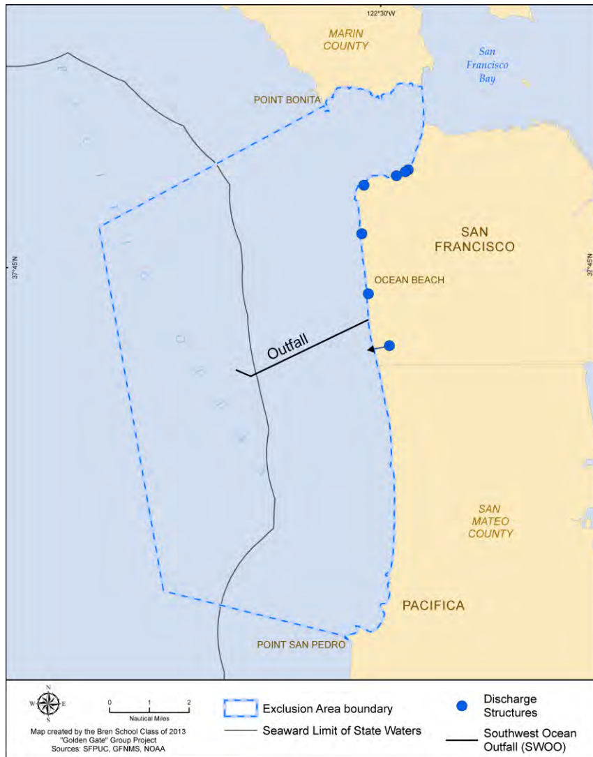
Figure 8: Wastewater infrastructure for San Francisco’s west side.
